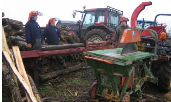
2 stages cleft oak stake processor
