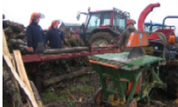
Fig 1: This is Coed Cymru's own construction: a cleft oak stake processor for small diameter logs. Several hundred logs can be processed per day. Furthermore, it is movable and easy to handle.
