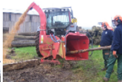
Fig 2: For the production of wood chips, used as fuel or for animal bedding, the Cilrhedyn Woodland Centre runs a wood chipper. Bigger offcuts or smaller and low quality logs are used for chip production. The machine is also transportable so the chip production can be carried out e.g. next to the shed where the chips are then stored.
