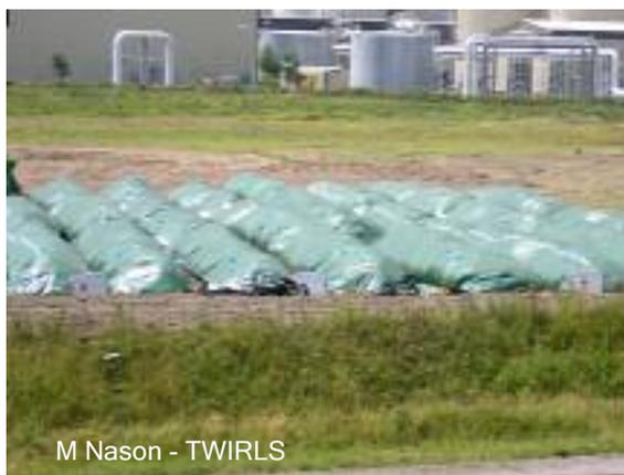
In the EcoPOD® system, a hydraulic ram pushes material from a feed-hopper into LDPE bags. A 60 m bag holds 100 m<sup>3</sup> of wastes aerated by perforated pipe connected to a fan.
